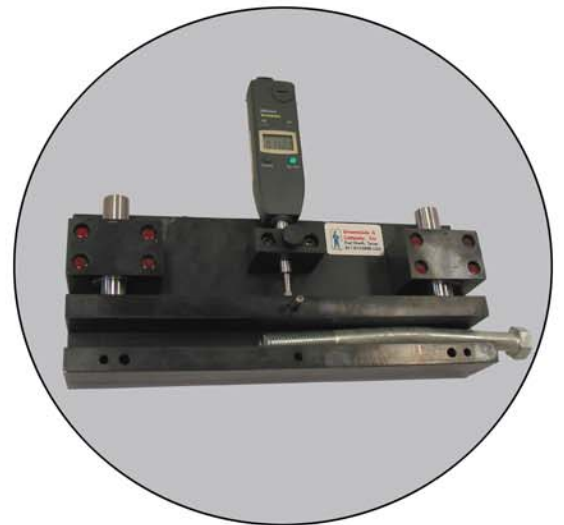
Step 2 - Bow of bolt turned to top of gage. Camber indicated on gage indicator.
